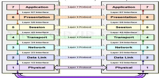
At each level (N), two entities (layer N peers) exchange protocol data units (PDUs) by means of a layer-N protocol. A service data unit (SDU) is the payload of a PDU, transmitted unchanged to a peer.
